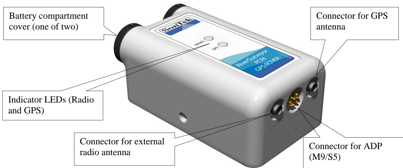
Figure 198. Configuration C – PCM RTK-GPS (Rover). The Figure shows the Rover PCM and its components. Note this is the same PCM as used for DGPS.
