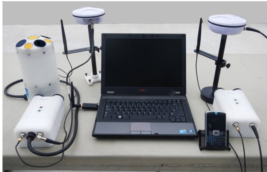
Figure 200. Configuration C – PCM RTK-GPS. Figure shows the different methods of connecting to the PCM: Via mobile phone (through Bridge (not pictured)), or through PC (via radio dongle on the left of the image). Figure also shows the GPS antenna with accompanying radio antenna and extension cord as well as the base station (typically mounted on a tripod as in the following figure).
