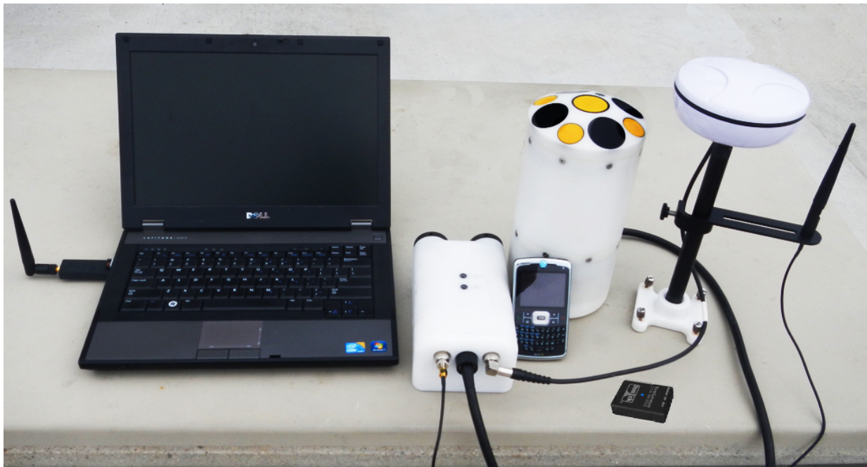
Figure 197. Configuration B – PCM DGPS. Figure shows the different methods of connecting to the PCM: Via mobile phone (through Bridge), or through PC (via radio dongle on the left of the image). Figure also shows the GPS antenna with accompanying radio antenna and extension cord.
