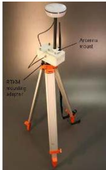
Figure 17. Hardware for the RTK Base Station
